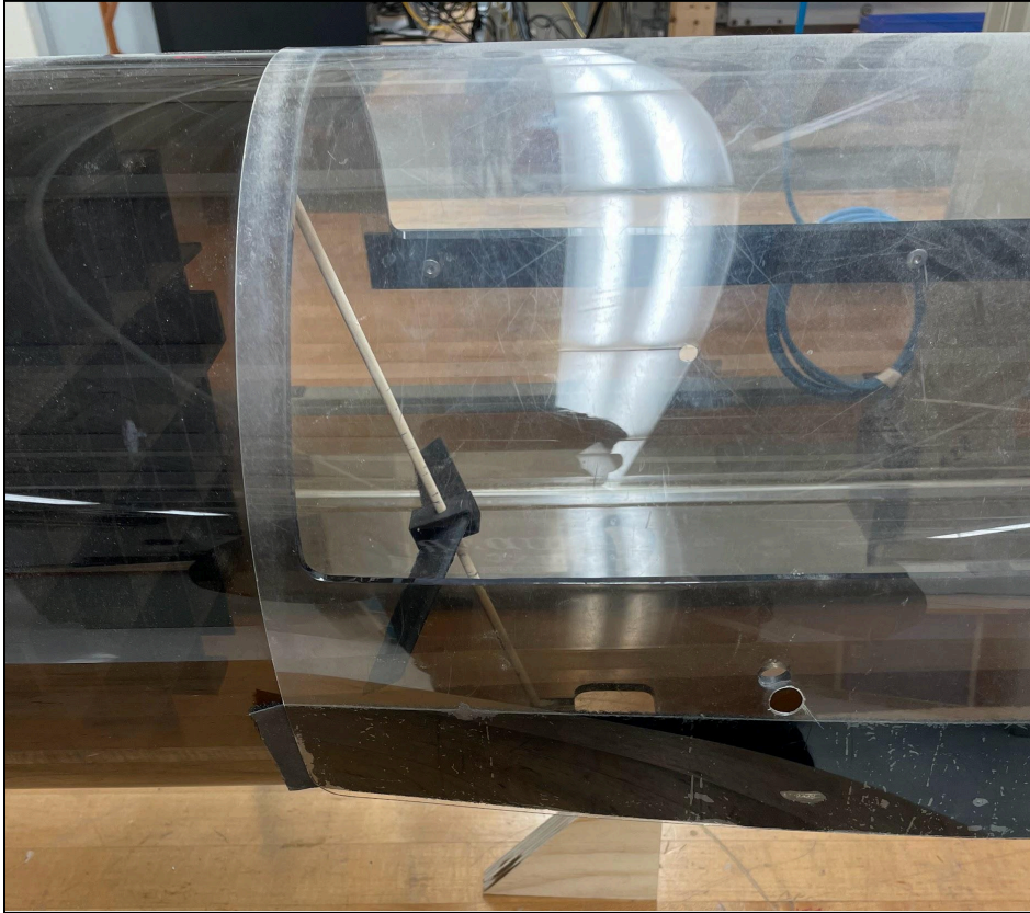
Figure 9. Wing Mount Setup in Wind Tunnel
